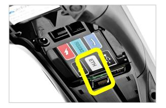
IMPORTANT: Do NOT plug the Ethernet cord into the RS232 port on the terminal
